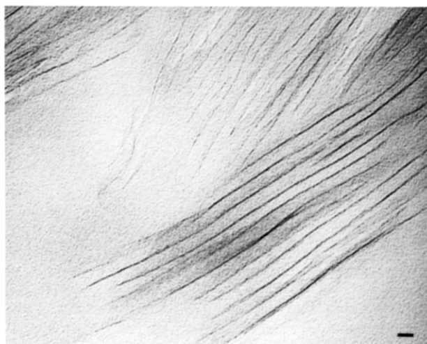
Figure 7. TEM micrographs of thin sections of fully cured OMTS/DGEBA/NMA nanocomposite containing 4% MTS by volume. Dispersed silicate layers are viewed edge-on and are clearly visible as dark lines of thickness approximately 10 Å, with 80–120 Å of epoxy matrix separating neighboring silicate layers. Scale bars = (a) 100 nm and (b) 10 nm.
